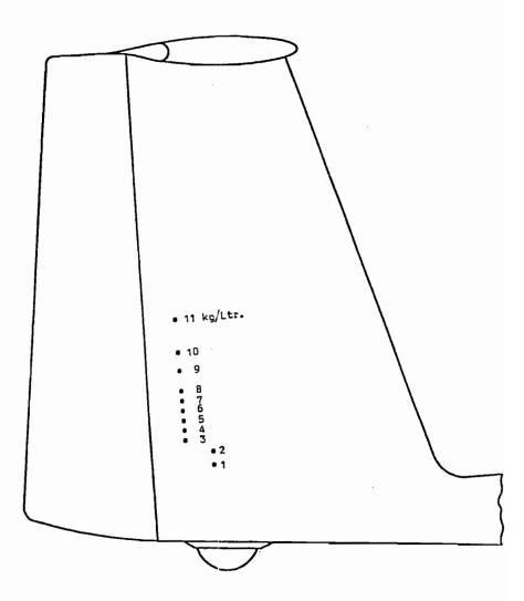
Water is dumped from the fin tank through an opening on the lower side of the fuselage tail boom - adjacent to the rudder.
